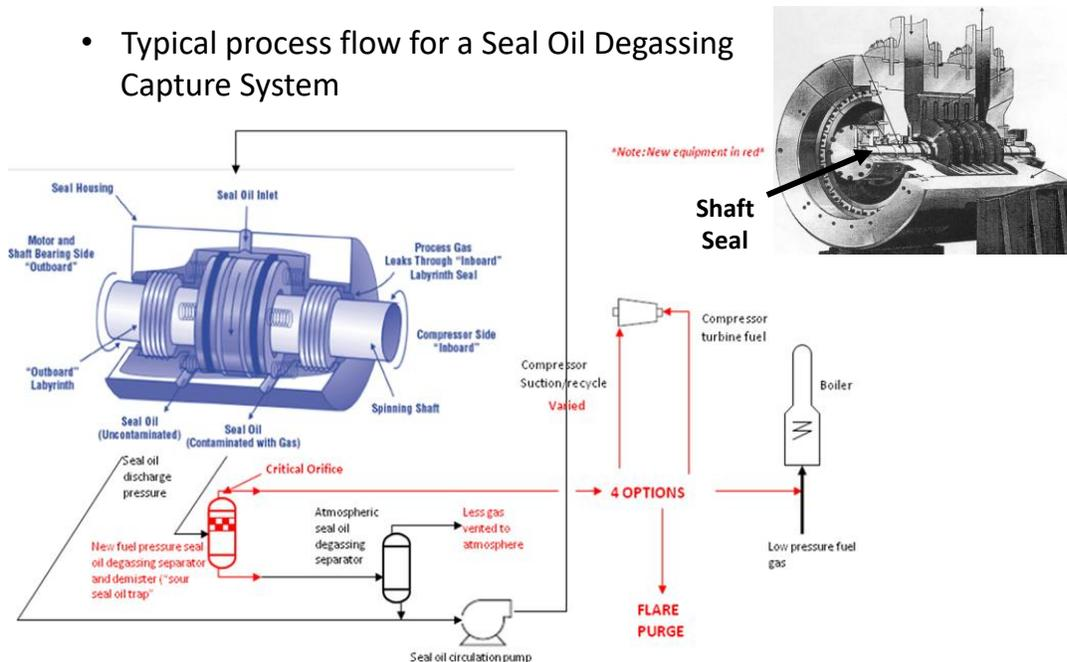
Reference: Natural Gas Star, *Wet Seal Degassing Recovery System for Centrifugal Compressors*, 2014
